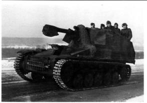
Left: The Wespe (Wasp), a 105mm gun-howitzer on a PzKpfw II chassis, was undoubtedly one of the most important - and one of the most numerous, self-propelled guns of the war. Some 682 PzIIs were converted to Wasps during 1943 and 1944 — mostly by a Polish firm in Warsaw. They saw wide service in the SP artillery battalions of panzer and panzergrenadier divisions. The one above was photographed in France during the winter of 1943/44.
