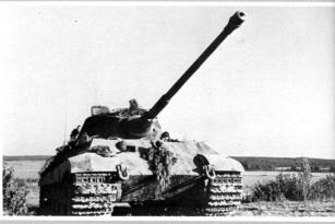
Right: The concrete like appearance of the armour surface was created by the application of a special paste to counter magnetic and sticky mines.
