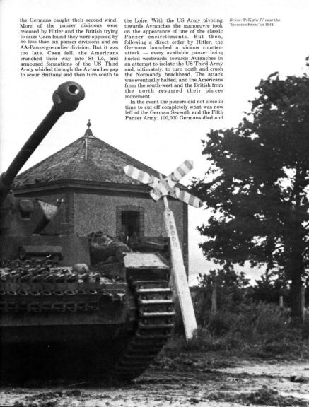
Right: PzKpfw IV near the 'Invasion Front' in 1944. Equipped with the L/48 75mm gun, and fitted with the Schürzen plates (skirting plates on the side for protection against infantry anti-tank weapons of the bazooka type).
