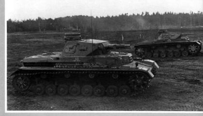
Above: The PzKpfw IV was originally designed as a medium support tank mounting a short 75mm howitzer. In the foreground is one of the early models on the Western Front in 1939. In the rear a PzKpfw III.
