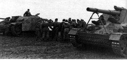
Above: An 'Orders Group'. Briefing before an operation besides two assault guns: Sturmgeschütz III Ausf. G (left) and Humme! (Bumble Bee) (right). The Humme! mounted a 150mm gun on a PX fpw IV chassis. Others were built on PZIII chassis.
