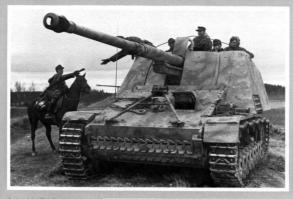
Left: The Nashorn (Rhinoceros) was a self-propelled anti-tank gun — mounting the ubiquitous S8mm PAK 43/1 L/71 gun on the chassis of a PaV. This photograph taken on the central sector of the Russian front early in 1944 suggests that the horse still had a communications role in a country of few roads and a shortage of PoL.
